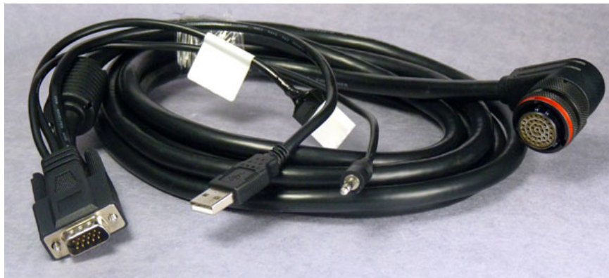
Figure 6. Photograph of a typical Monitor Power and Signal Cable, with standard PC-compatible connectors (DB15 for video, USB for touch screen and 3.5mm for audio). It also has a 4-pin 3.96mm Socket for DC power.
